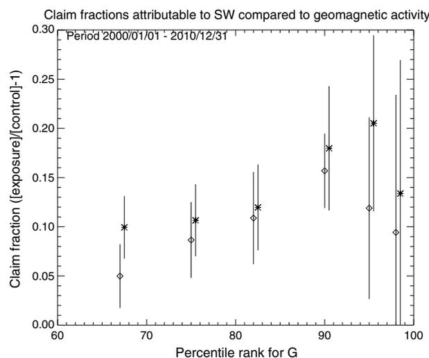
**Figure 7.** Relative excess claim frequencies statistically associated with geomagnetic activity (difference between claim frequencies on geomagnetically active dates and the frequencies on control dates as shown in Figure 5, i.e.,  $(n_i - n_c)/n_c$ ) for the full sample (*A*; diamonds) and for the sample (*B*; asterisks) from which claims were removed attributable to apparently nonspace weather-related causes.
