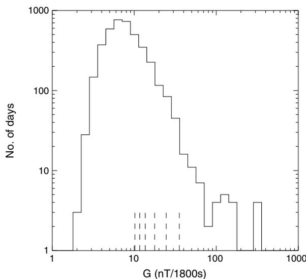
**Figure 3.** Histogram of the number of days between 1 January 2000 and 31 December 2010 with values of  $G \equiv \max(|dB/dt|)$  in logarithmically spaced intervals as shown on the horizontal axis. The 98, 95, 90, 82, 75, and 67 percentiles (ranking  $G$  from low to high) are shown by dashed lines.
