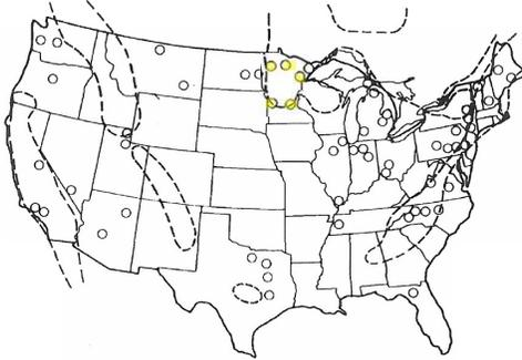
Figure 1. Locations of GIC Recorders on Power Systems from 1969-1972 (Indicated by Circles). Dotted Lines Outline Areas of Igneous Rock Geology.
