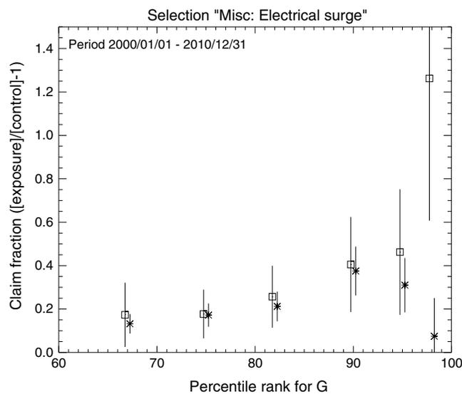
**Figure 8.** Same as Figure 7 but for sample *B* limited to those claims attributed to “Misc.: Electrical surge” (asterisks) (for 57% of the cases in that sample), compared to the fraction of high-voltage power grid disturbances statistically associated with geomagnetic activity (squares).
